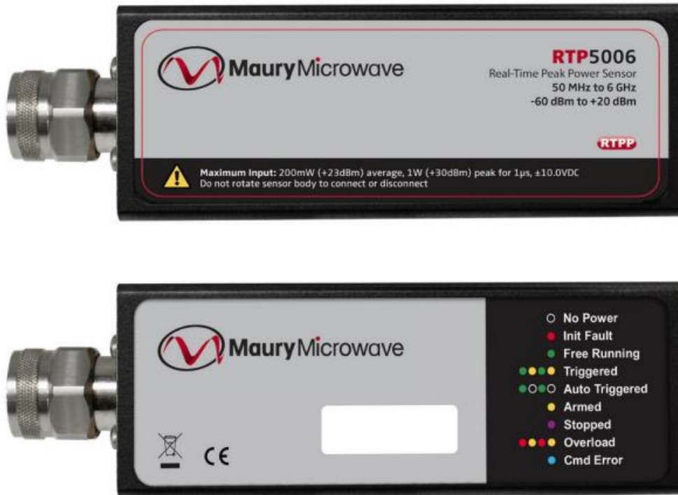
Figure 2.6 The information labels on the RTP Series Real-Time Power Sensor contain information on the maximum power levels the device can handle and the meaning of the various status LED flash patterns.
